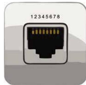
The battery communication interface adopts 8P8C RJ45 socket.
