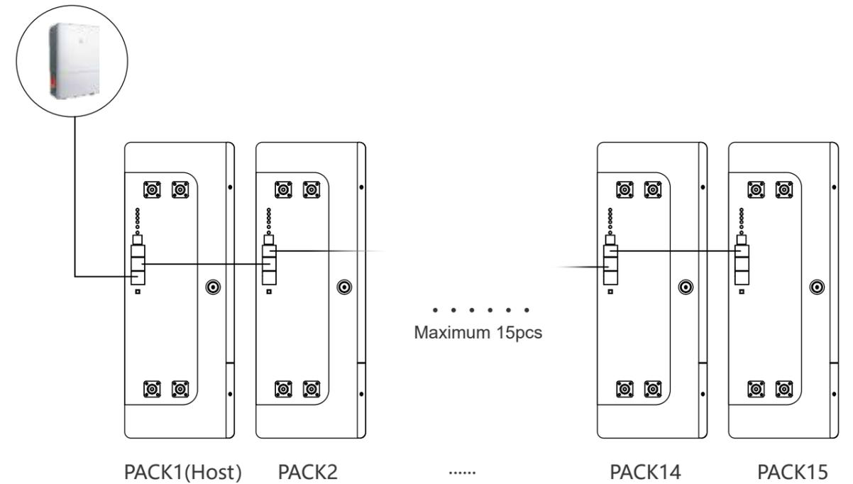
④ Batteries are connected in communication
