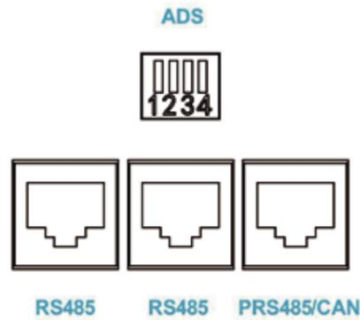
“ADS” is used for parallel use of battery packs. PACK can be distinguished by hardware address. The definition of ADS master-slave address refers to communication address selection specification. “PRS485/CAN” battery pack can communicate with the upper computer or inverter and the reverse control integrated machine through the interface. “RS485” is used in parallel for battery pack, and the main communicates with pack from the interface.
