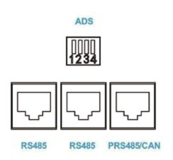
"ADS" is used for parallel use of battery packs.
