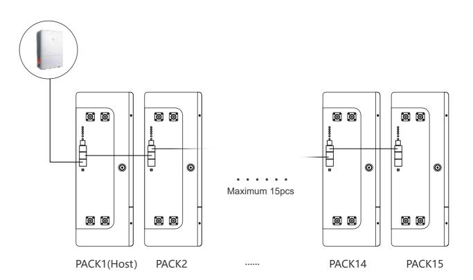
4 Batteries are connected in communication
